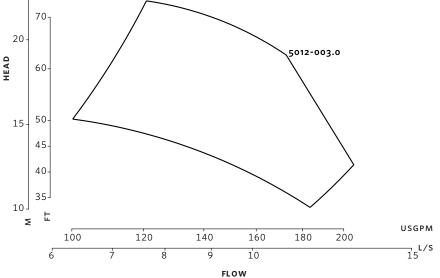
INDOOR (IP 55/TEFC) Size: 50-125 **κW:** 3.0 **RPM:** 3600 **AB:** 457 (18.01) **B:** 109 (4.31) 88 (3.46) c: 154 (6.07) D: **E:** 191 (7.54) 180 (7.07) s: 334 (13.14) SD: **T:** 79 (3.12) Weight: 36.7 (81)
