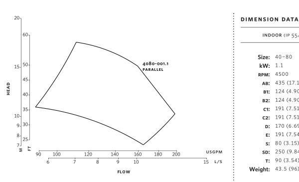
INDOOR (IP 55/TEFC) **Size:** 40-80 **kW:** 1.1 **RPM:** 4500 435 (17.14) AB: **B1:** 124 (4.90) **B2:** 124 (4.90) **c1:** 191 (7.51) **c2:** 191 (7.51) D: 170 (6.69) 191 (7.54) E: s: 80 (3.15) **sp:** 250 (9.84) **T:** 90 (3.54) Weight: 43.5 (96)
