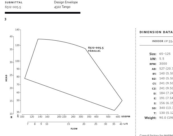
INDOOR (IP 55/TEFC) Size: 65-125 **kW:** 5.5 **RPM:** 3000 **AB:** 527 (20.75) **B1:** 140 (5.50) **B2:** 140 (5.50) 241 (9.50) C1: **c2:** 241 (9.50) **D:** 184 (7.24) **E:** 191 (7.54) s: 156 (6.15) **sp:** 340 (13.39) **T:** 130 (5.12) Weight: 90.0 (198)
