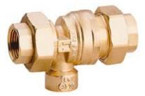
BFP series valves include two spring-loaded check valves that act independently for positive protection, and also have an intermediate atmospheric vent that ensures a safeguard against backflow conditions.
