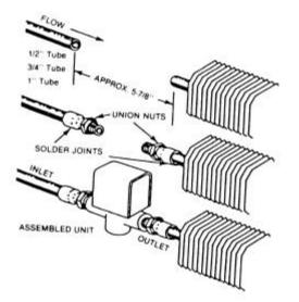
AMZI valves are machined to accept the fittings shown. This type of connection eliminates the need for precision cut lengths of copper tube. Close quarter fittings make connection easy without tube benders or flaring tools.
