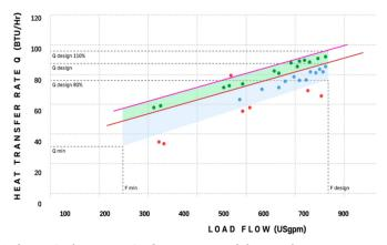
Adept Selection Software enables selection of the Systems Envelope - Energy Transfer Station in minutes, optimizing components for the lowest first and operating costs.
