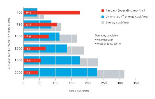
Retrofit projects that improve HVAC efficiencies pay back the costs of the project over time through energy savings. Depending on the existing efficiency levels and cooling profile of a building, installation of an OPTI-VISOR™ can save enough energy to generate a payback on the project cost in less than one year.
