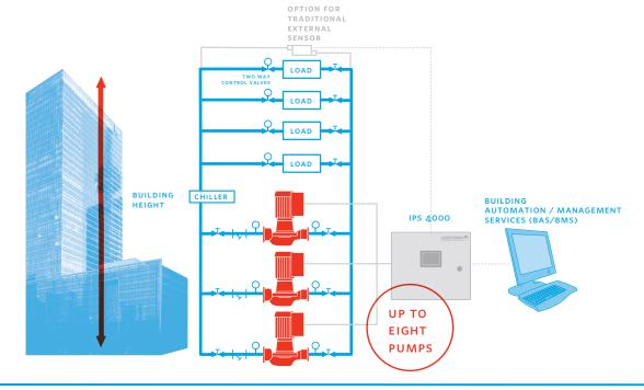
Armstrong Design Envelope pumps are equipped with Sensorless Technology and do not need external sensor to satisfy the HVAC load demand. Parallel Sensorless technology in the IPS optimizes pump operation to use the lowest possible pump energy.
