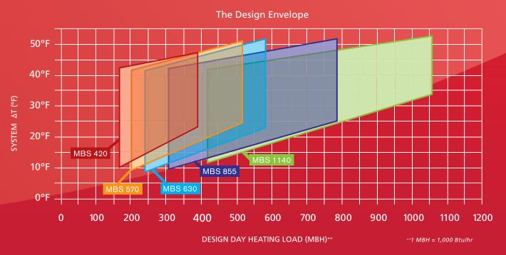
The operating envelopes of the ECO\*PAK MBS are able to achieve efficiencies of over 90% because the heat output constantly matches the actual building load demand.
