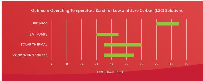
If we are to get the best out of our LZC (Low and Zero Carbon) solutions we can't look at each of them in isolation. If they are to work together in the same system, they need to be fully integrated so that the conflict between the different operating temperature ranges is effectively managed.
