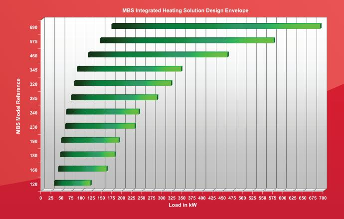
The operating envelopes of the MBS Integrated Heating Solution are able to achieve overall seasonal efficiencies of over 90% because the heat output constantly matches the building load.
