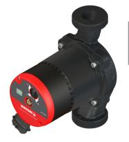
TECHNICAL DATA up to  $4.4 \text{ m}^3/\text{h}$ Rate of flow: Pressure head: 4 m/6 m/8 m 4-20 W/5-37 W/6-64 W Control range: Media temperature: +2 °C to +110 °C Installation length: 130 and 180 mm Threaded connection: 1", 11/2" and 2" Protection class: IP 42 Insulation class: Nominal pressure: PN 10 Control:  $\Delta pc + \Delta pv + fixed rpm$  $\leq$  0.17 HEP Optimo XX-4.0 GXXX EEI:
