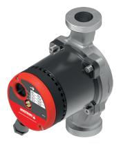
TECHNICAL DATA Rate of flow: up to 4.0 m<sup>3/</sup>h Pressure head: up to 6 m Media temperature: +2 °C to +110 °C Installation length: 130, 150 and 180 mm Threaded connection: 1", 11/4" and 11/2" Protection class: IP 44 Insulation class: Н Nominal pressure: PN 10 Control: 3-step switch with manual speed selection
