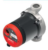
TECHNICAL DATA Rate of flow: up to 12.0 m<sup>3</sup>/h Pressure head: up to 12 m Media temperature: +2 °C to +110 °C Installation length: 180 mm Threaded connection: 11/4" and 11/2" IP 44 Protection class: Insulation class: Н PN 10 Nominal pressure: Control: 3-step switch with manual speed selection
