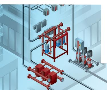
Because HVAC pumping systems mostly operate at partload, a design using two or more smaller pumps is more efficient than one larger pump. In a two-pump system, if one pump fails, the remaining pump can serve the system requirements with up to 70% flow redundancy. The capacity split can be adjusted based on the building type and duty requirement.
