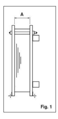
'A' for 032 plates = total number of plates x 2.9mm 'A' for 150 plates = total number of plates x 2.5mm
