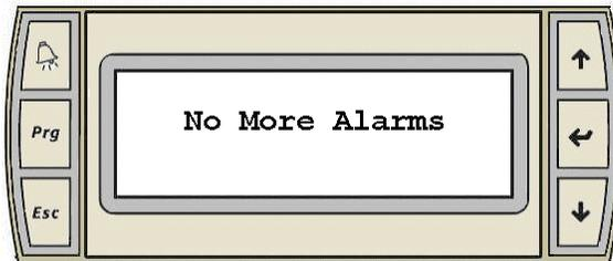
3. This display will also appear when navigating through a number of Active Alarm displays to indicate when you reach the end of the list of active alarm.
