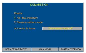
1 Where if Commission mode off/on switch is in Commission mode on position it disables the no flow shutdown and the pressure setback mode. The commission mode is active for only 24 hours. The commission mode is used for testing an IVS Booster system in case of not occupy building with no flow in it.
