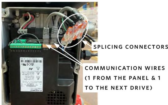
**2** Insert the RJ45 Header into either RJ45 port in the drive. The ports are wired in parallel so either port will work.
