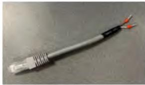
**FIGURE 2.2:** Splicing Connector
