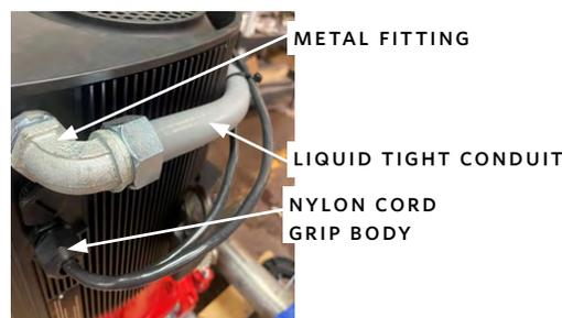
**NOTE:** We need to attach the metal fitting and nylon cord connector to the new motor, so keep them safely stored away.
