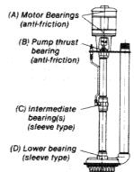
(A)/(B) The motor bearings and pump thrust bearing are pre-lubricated and sealed. No further lubrication is required during the life of the bearings.
