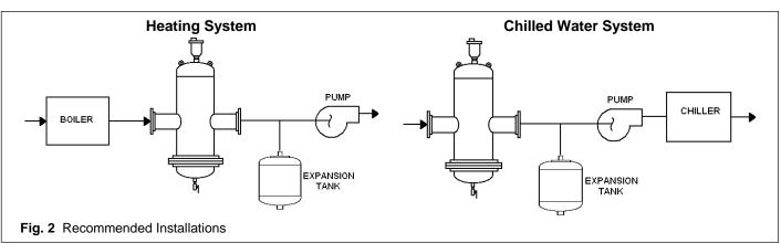
Note: 100% of system flow should pass through the DAS to ensure all particles can be filtered.
