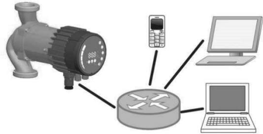
Figure 5: connecting to a network via router
