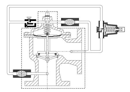
The dashed line seperates the internal main body valve and the external pilot assembly.
