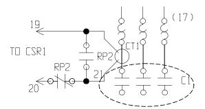
Contacts (RP2) close to start the motor running or open to shut one down. This action opens or closes the motor contactors (C1).
