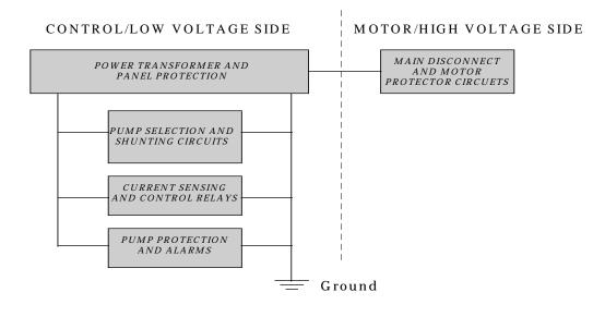
Block Diagram of Complete Control Circuit
