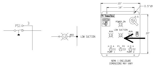
Fig.# 21: Low suction pressure switch shuts down system and warns by lighting pilot.
