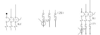
The short circuit protector (left) and overload protector (middle) combine to form a complete motor protector circuit (right). Within the controller, these components are integrated into a single component called an overload relay. The device has a setting for the maximum allowable amperage, and a two push button circuit breaker (pushing in the red button opens the circuit / pushing in the white button closes the circuit).
