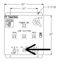
Manual alternator switch determines which pump leads.
