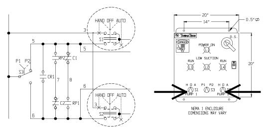
Pump Shunting Circuit holds key to pump sequencing. The circuit is only activated when the pumps are placed in the AUTO position.
