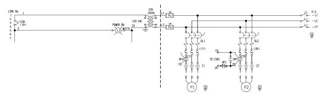
Control Protection, Transformer and Motor Protector Circuits. The portion of the schematic on the left side of the dashed line was discussed in this section.
