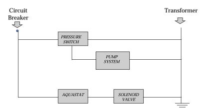
Block Diagram of Pump Protection Circuit
