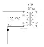
Control Transformer. The left side is the low voltage side providing power to the panel. The right side is the high voltage supply which powers the motors.
