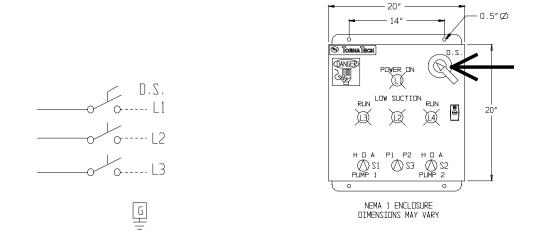
Schematic of Disconnect Switch. The location of the switch on the panel is indicated by the arrow.
