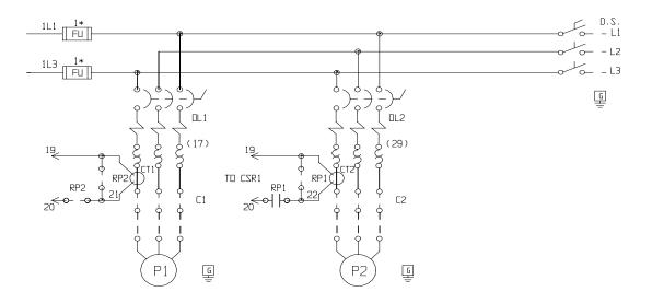
Main Disconnect and Motor Protection Circuit. Note that the lower segment of the diagram (marked "P1" and "P2") represents the motors and their respective starters.
