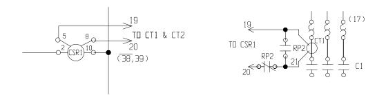
Current Sensing Relay. In combination with a control relay, the CSR activates a current transformer in the starter (part of the contact arrangement) to start the motor. The numbers 19 and 20 marking the arrows indicate a connection to the matching numbers on the motor lead. TIP: The number of current sensing relays in a system can be determined by the formula:
