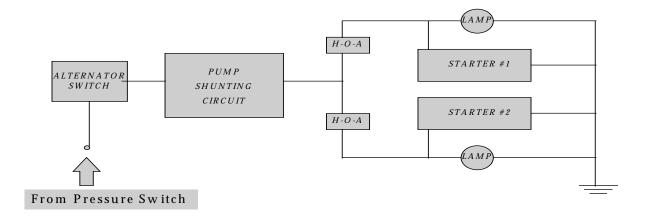
Block Diagram of Pump Selection and Shunting Circuits
