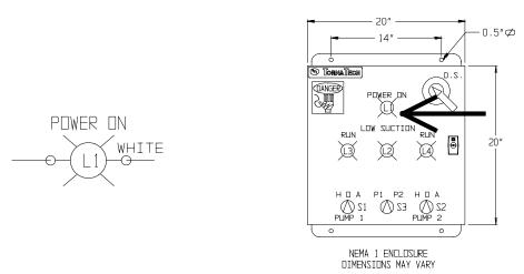
The Power On pilot light informs the controls operator that the panel is live.
