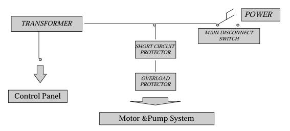
Block Diagram of Main Disconnect and Motor Protector Circuits
