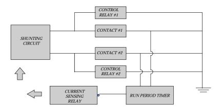
**Current Sensing and Control Relays**
