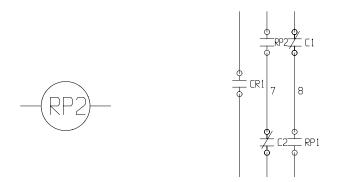
Control Relay Coil actuates the motor starter contacts inside the shunting circuit.
