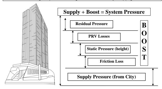
Relationship of Boost Pressure vs. System Pressure. <u>Boost Pressure</u> is what we design for. <u>Supply</u> <u>pressure</u> is that which is currently available. Combined, these form <u>System Pressure</u>.
