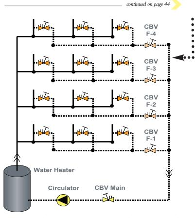
Without recirculation system balancing, the most disadvantaged branch would receive the least flow, whereas the most advantaged branch would receive the majority. Unless the system is balanced, hot water users on the most disadvantaged branch would still have I ong wait times.
