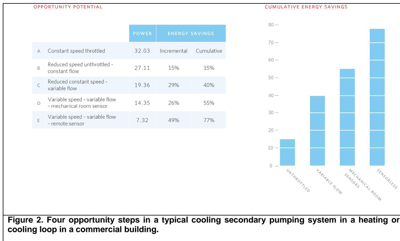
**Figure 2. Four opportunity steps in a typical cooling secondary pumping system in a heating or cooling loop in a commercial building.**
