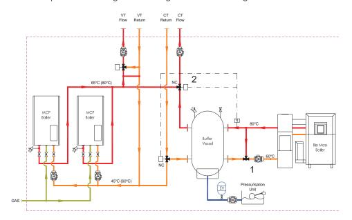
An example of an integrated design is shown in figure 12.
