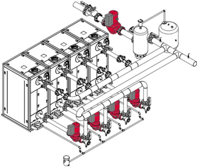
Boiler circulation pumps circulate water within the boiler to enhance boiler operation and influence the overall efficiency of the system.
