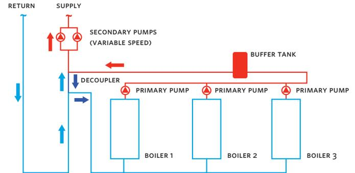
The figure shows a typical constant primary variable secondary system consisting of three boilers running in parallel each having its own circulating pump. The Decoupler, decouples or 'hydraulically separates' the primary (boiler) and secondary (system) loops and prevents flow in one circuit from interfering with the other. Hence as zone valves open, close, or modulate, and as system pumps vary speed, the boiler loop is not impacted.
