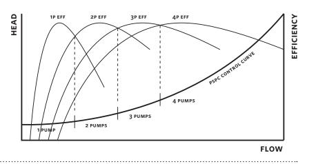
chieving coordinated, parallel operation is a key step in reaching peak efficiency levels in pumping systems that employ multiple units. Digital control technology made available in the last 10 years has made this possible, and the use of variable speed drives to control pumps is now an established practice.
