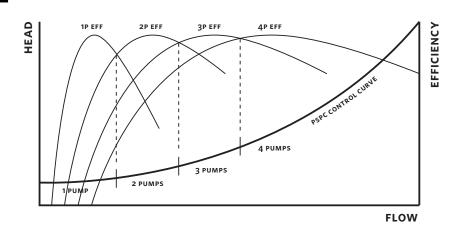
chieving coordinated, parallel operation is a key step in reaching peak efficiency levels in pumping systems that employ multiple units. Digital control technology made available in the last 10 years has made this possible, and the use of variable speed drives to control pumps is now an established practice.
