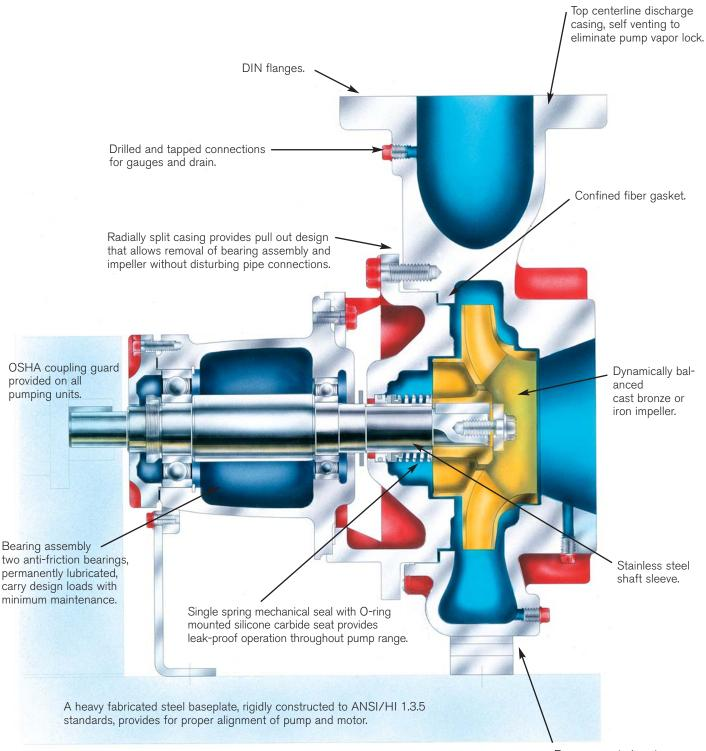
Base supported casing eliminates need to support casing when bearing assembly is removed.
