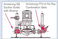
Vertical In-Line with Suction Guide and Flo-Trex valve eliminates cost and space of all the items listed under base mounted pump, plus the following:
