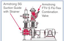
Base mounted pump with Suction Guide and Flo-Trex valve eliminates cost and space of:
