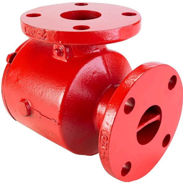
**A**rmstrong Suction Guides are installed on the suction side of pumps to protect against damage from debris and foreign matter, and to optimize flow efficiency. Most pump installations require a long-radius elbow, flow-straightening entrance pipe, and Y strainer. The Suction Guide's versatile 4-function design saves space and installation costs by incorporating all these devices into a single solution.
