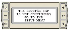
• When the booster has not been setup this display and the main menu display will be the only operation displays to appear.
