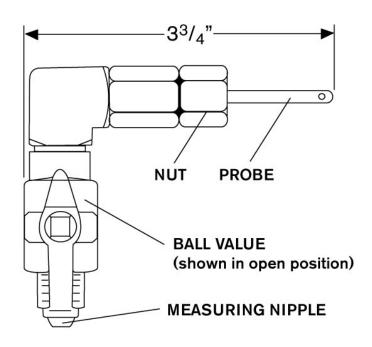
FOR USE ON ALL CIRCUIT BALANCING VALVES WITH P.M.P. METERING PORTS AND ARMSTRONG METERS: CBDM-60, CBDM-135/60, APDM-135/60 WITH SCHRADER FITTINGS.
