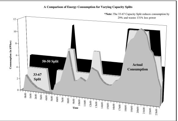
Notice that by simply changing the flow split percentages, the pumps now follow the system demand more accurately. This is how to optimize power consumption with constant speed pressure booster packages. The system becomes, in essence, a variable flow package, choosing the best motor (or combination of motors) to run for a given GPM.
